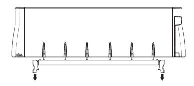
**8.3** Pull Arm and Lines horizontally forward from the cabinet towards the Receiving Bracket.
