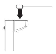
8.5 Seat the Arm within the Receiving Bracket. Allow the Arm and Lines to slide back towards the cabinet and engage on the two Locking Pins within the Receiving Bracket.
