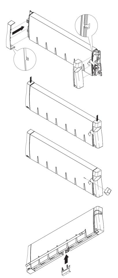
Before you mount the Receiving Bracket there are a couple of quick steps to follow to expose the mount holes.
