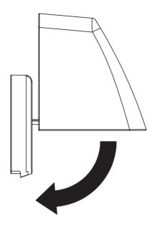
7.2 Align the Outer Cover internal slots with Backing Plate outer ribs. Slide the Cover onto the Backing Plate and allow the Cover to return to the top position. Jiggle the Cover to free it should it not slide smoothly.
