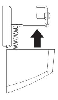
**7.3** Push the Cover downward and allow it to spring upward to test its operation.
