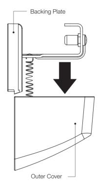
**5.3** Rotate the Outer Cover upward to expose the mount holes.
