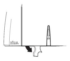
**8.2** Pull Arm and Lines downward from the cabinet using the Arm Handles.
