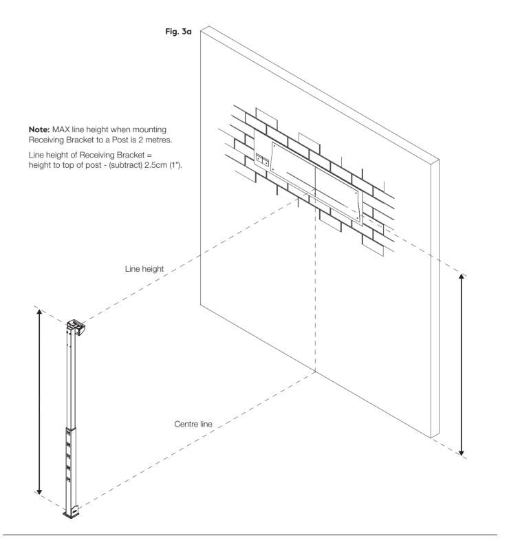
**3a.5** Masonry fasteners are not included with this product. When attaching to a sound masonry wall, 5 x 10mm (13/32") diameter masonry sleeve anchors are recommended.
